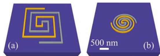
FIG. 1. Schematic representation of the proposed Seebeck nanoantennas: (a) a square spiral and (b) an Archimedean spiral. These geometries consist of two symmetrical arms made of dissimilar metals, what creates a thermocouple. For each arm, the cross section is 200 nm width \times 100 nm thick. Substrates consist of 1.2 \mu\text{m} thick \text{SiO}_2 layers.
